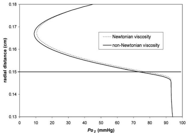
Figure 6. Radial  $P_{O_2}$  profile at the location of flow reattachment with Newtonian and non-Newtonian blood viscosity. Flow rate = 180 ml/min. Oxygen consumption in the wall =  $1.3 \times 10^{-4} \text{ ml./ml.tissue-sec}$ . The wall thickness is 300 micron.
