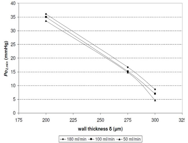
Figure 5. Variation of  $P_{O_{2,min}}$  for variable  $\delta$  at  $z = 7 \text{ cm}$
