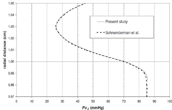
Figure 2. Comparison between results obtained by the present study and those obtained by Schneiderman et al. [11] using same geometry, properties and boundary conditions
