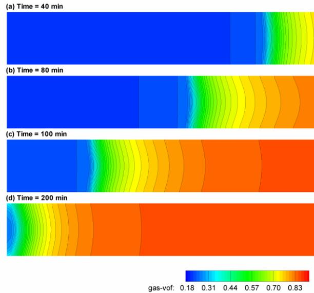
Figure 9. Methane gas saturation contours at different times.
