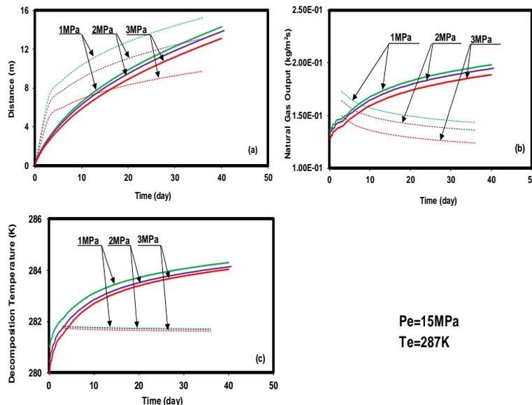
**Figure 4.** Comparison of present time variations of the position of dissociation front, natural gas output and dissociation temperature with linearized solutions for different well pressures. Solid lines: numerical solutions; Dashed lines: linearized solutions suggested by Makogon (Ji et al., 2001).
