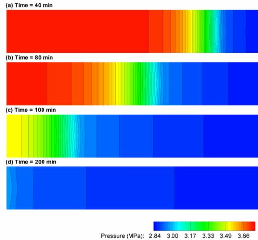
**Figure 6. Pressure contours in the core sample at different times.**
