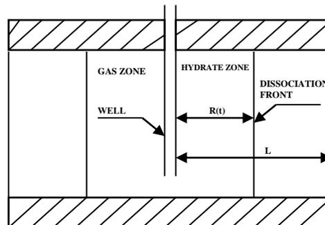
Figure 1. Schematics of the hydrate reservoir for the axisymmetric model.
