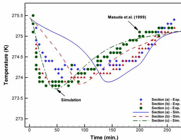
Figure 10. Comparison of temperature variations from simulation to experimental data.
