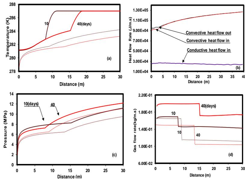
**Figure 3. Comparison of the present temperature and pressure profiles and mass flow rate with linearized solutions for a reservoir temperature of 287K and a well pressure of 2MPa. Solid lines: numerical solutions. Dashed lines: linearized solutions suggested by Makogon (Ji et al., 2001).**
