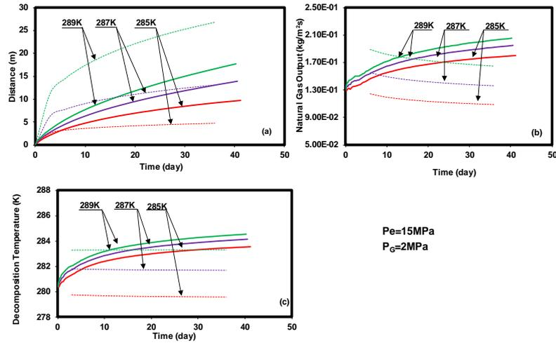
Figure 5. Comparison of the present time variations of the position of dissociation front, natural gas output and dissociation temperature with linearized solutions for different reservoir temperatures. Solid lines: numerical solutions; Dashed lines: linearized solutions suggested by Makogon (Ji et al., 2001).
