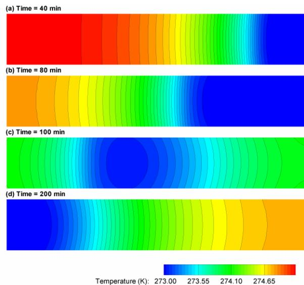
**Figure 7. Temperature contours in the core sample at different times.**
