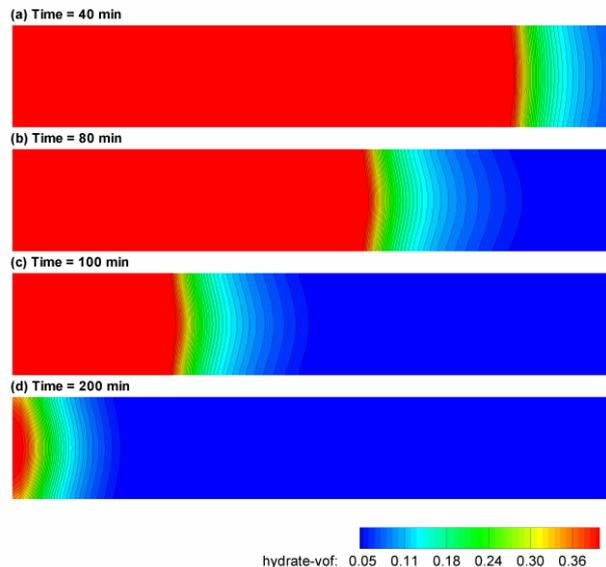
**Figure 8. Hydrate saturation contours at different times.**
