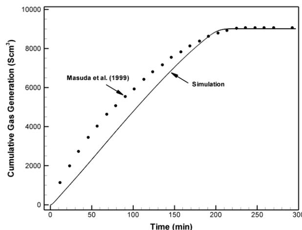
Figure 11. Comparison of cumulative gas generation with the experimental data.
