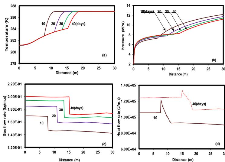
**Figure 2.** Time variations of pressure, temperature, gas mass flow and heat flow profiles in a reservoir for a well pressure of 2MPa and a reservoir temperature of 287K.
